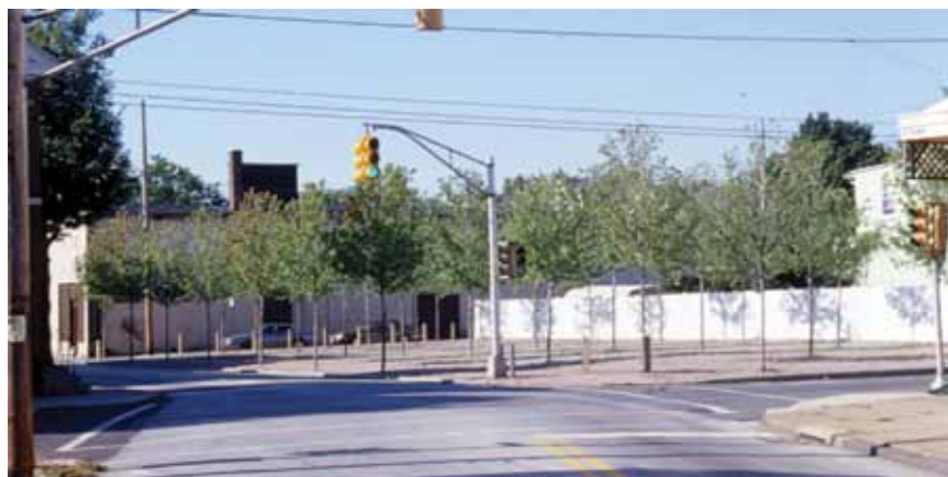
The asphalt was removed and 35 red maple trees were planted in two feet of topsoil with a crushed stone surface.
