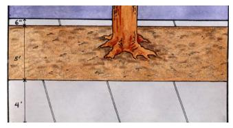
Tree pits can be expanded by removing excess concrete to form a planting strip to allow tree roots space to grow and reduce the chance of a lifted sidewalk. It also allows rain to permeate the ground.
